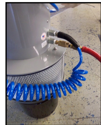
Straight hose supplies the MiJET with compressed air.
